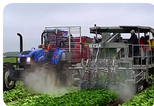
Taylor Farms uses a high-pressure water jet harvester on a portion of their lettuce crop.
